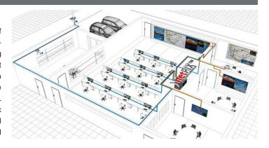
The netPIX-core controllers provide multiple analog and digital video and graphic connectivity with input cards. Thanks to latest Switch Fabric architecture, video and graphic sources can be displayed simultaneously on the display wall in full frame rates. All analog and digital Video-/RGB-/DVI- and IP Streaming data is transmitted with up to 192 GB/s without any dependencies on the system.
